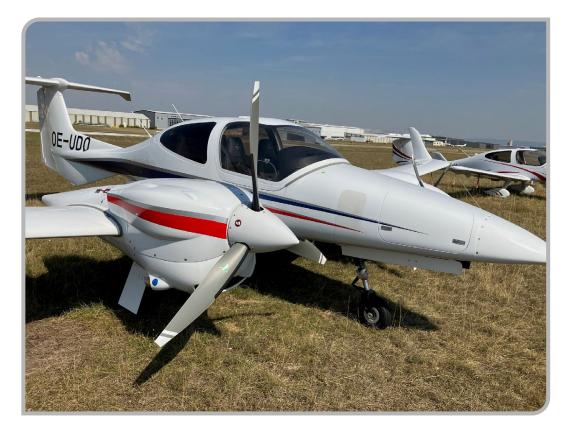
ENGINES Two Austro Engine 168HP AE300 Turbocharged Common-Rail Injected 2.0 Liter Diesel Engine and EECU Single Lever Control System
