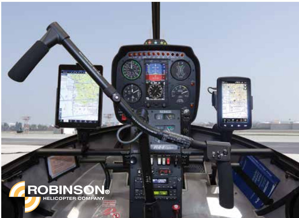
Six-hole instrument panel shown with optional Aspen EFD1000H, Spidertracks, and dual accessory support bars with mounts (Apple iPad and Garmin GPS not included).
