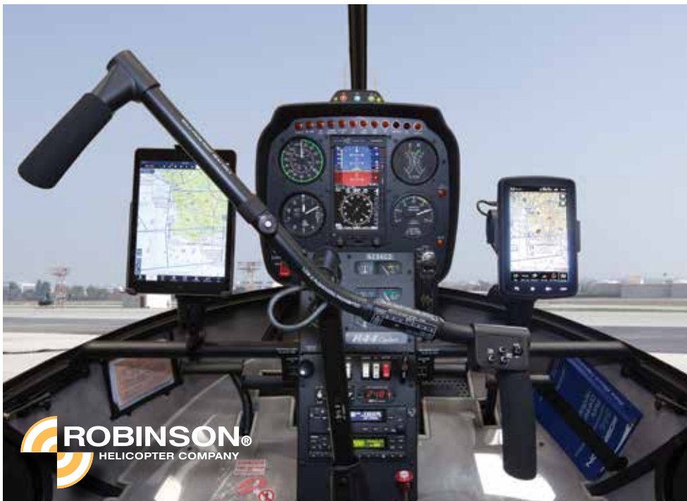
Six-hole instrument panel shown with optional Aspen EFD1000H, Spidertracks, and dual accessory support bars with mounts (Apple iPad and Garmin GPS not included).
